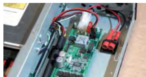
The latest DC to DC power adaptors avoid the use of inverters and mains voltages. Developed for commercial trucks, they are over 95% efficient and have high input ranges 6v to 32v for reliable 12v or 24v operation.
