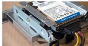
Industrial shock mounts fitted to conventional hard drives
