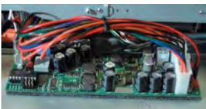
The latest DC to DC power adaptors avoid the use of inverters and mains voltages. Developed for commercial trucks, they are over 95% efficient and have high input ranges 6v to 32v for reliable 12v or 24v operation.
