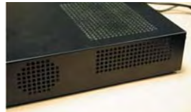
Ventilation holes required for cooling but filters added for models with a fanned processor
