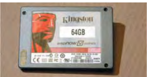
Solid state hard drive - no moving parts to break or skip
