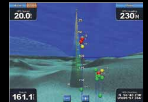
Fish Eye 3D Underwater perspective view shows fishing target detected by connected GSD 22 sonar.
